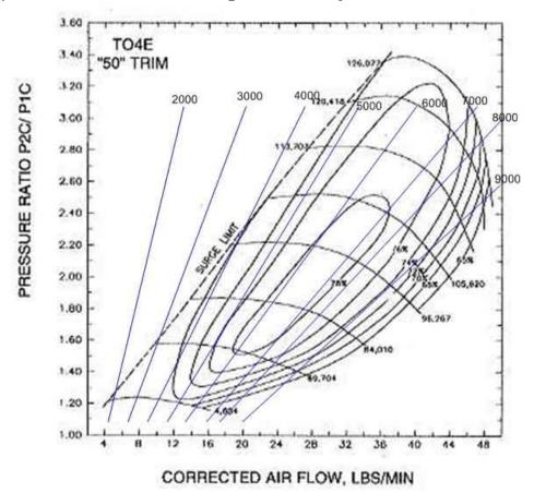
The T04E 50 trim has been used successfully to make over 400 hp at the crank at around 20 psi on various MR2T's. This plot shows that this turbo, while a bit larger, will be very happy in the rpm's surrounding redline, assuming a stock level near 7500 is being utilized.
